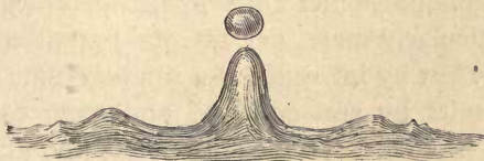
Fig. 223.—Ex.—Ejection of Drop upon Recoil from Surface of Water. (Enlarged 1\frac{1}{2} diameters.)
